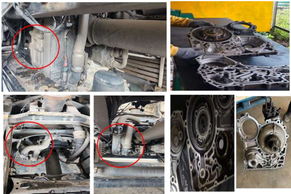
Figure 9. Retarder Replacement Source: Researcher Documentation at PT XYZ, 2025
